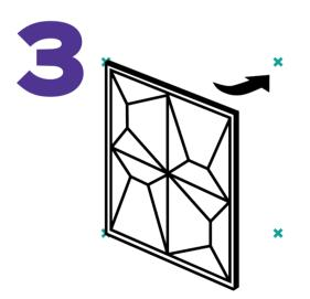
Carefully place the tile following the marked points, strating from one side.
