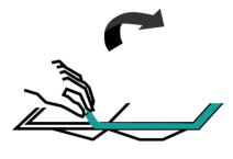
Remove the outer layer of the assembly tape attached to tile's back frame.
